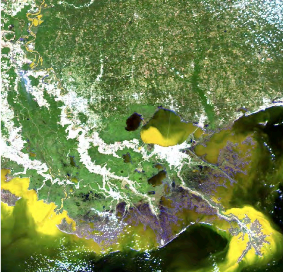
USGS satellite image of the lower Mississippi River basin during the 2011 flood; sediment plumes are shown in yellow; the intense yellow plume in the center is in Lake Pontchartrain, channeled through the Bonnet Carre Spillway.
