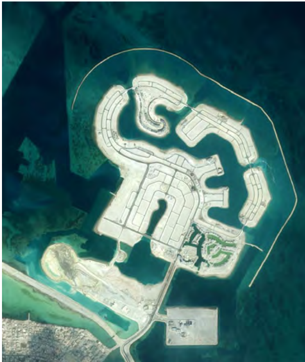
Aerial view of Amwaj Island, Bahrain. As described by Geotec Associates, "The key element in the successful design, construction and completion of the Amwaj Island development project was the use of sand filled Geotubes to form the island perimeter for containment of 12 million cubic meters of dredged sand that formed the basic platform for the development project. The island perimeter was constructed by hydraulically filling Geotubes with local sands from proposed navigation channels and marinas serving residents and businesses on the main island of Bahrain...Amwaj Island development will provide a variety of amenities such as living in beach front properties, hotels, restaurants, recreation parks, theaters, marinas, and golf courses." 11
